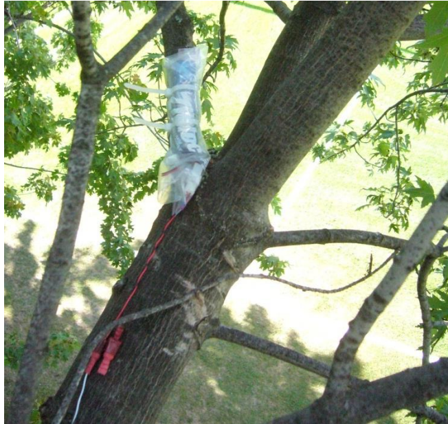
Fig. 1 Typical accelerometer installation
